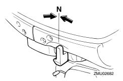
2. Slightly tilt the outboard motor up until the tilt support bar automatically turns to the lock position to support the engine.
